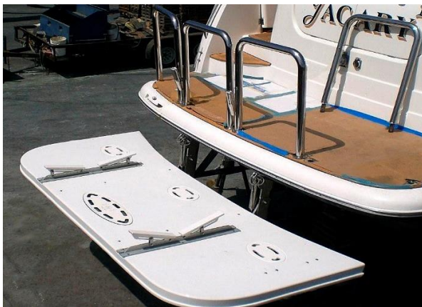
Fig. 10 Hydraulic platform being installed (note chocks)
