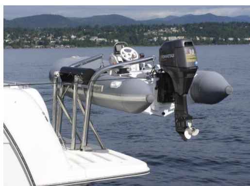
Fig. 2 Marlin board mounted davits #1
