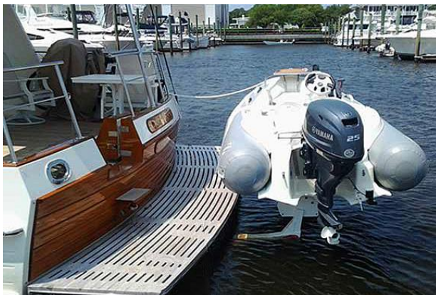
Fig. 8 Lift 'Cradle' underneath marlin board #1
