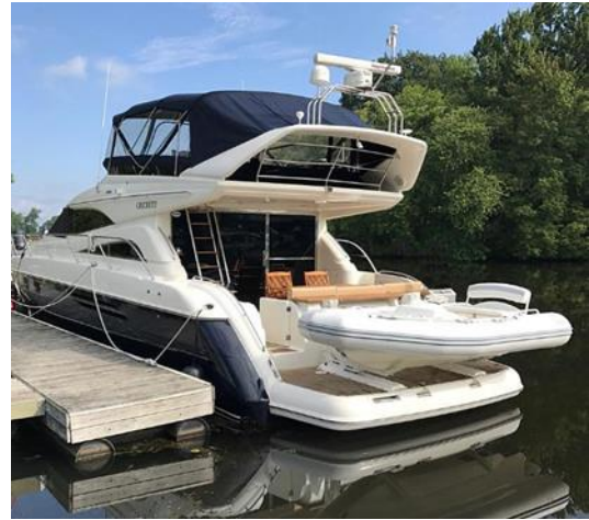
Fig. 17 PM XL500 Raillift on deep platform/deck
