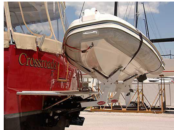
Fig. 9 Lift 'Cradle' underneath marlin board #2
