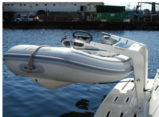
Fig. 3 Marlin board mounted davits #2
