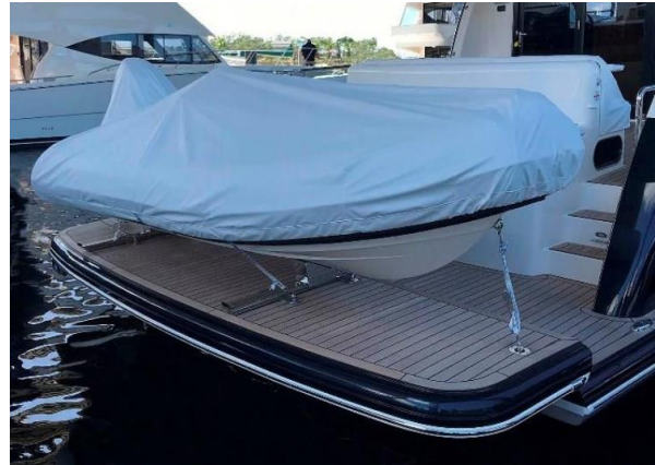
Fig. 11 Hydraulic Platform with Tender Secured
