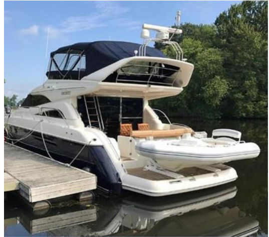
Fig. 15 XL500 Rail Lift on Deep Platform/Deck
