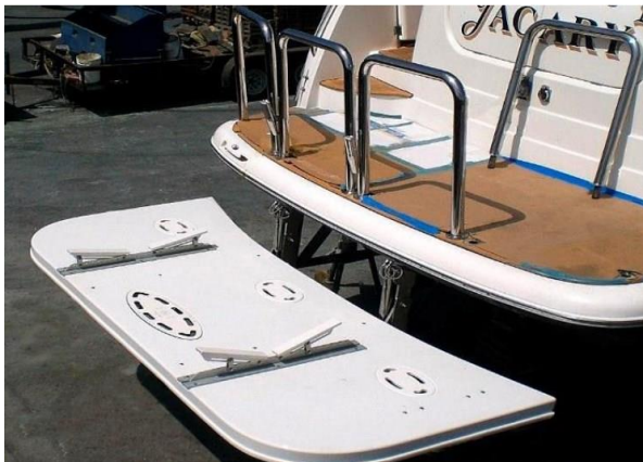
Fig. 10 Hydraulic Platform Being Installed (note chocks)
