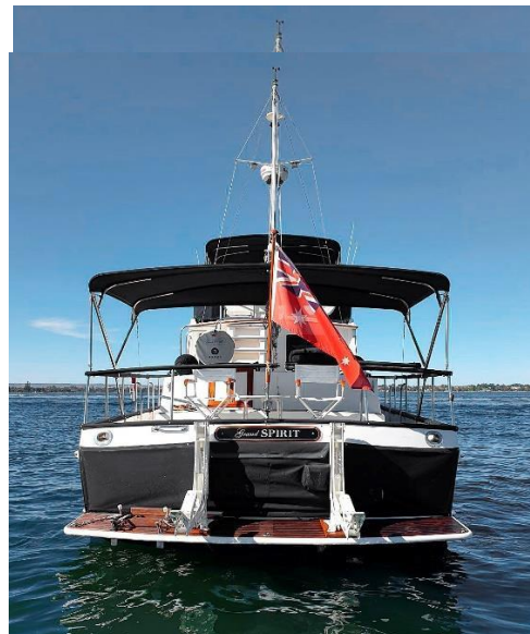
Figure 13: Lift fitted onto the existing swim platform of my Grand Banks 42 Classic.
